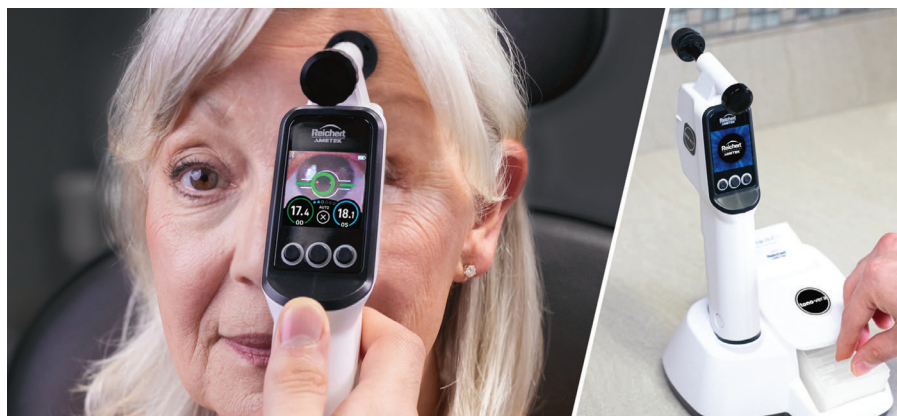
The Reichert Tono-Vera uses ActiView Positioning to find the corneal apex.
